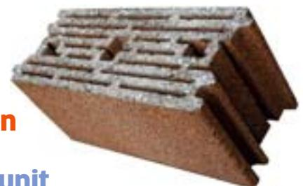
Eurobéton Industrie (Building Distribution) has developed a new expanded clay concrete masonry unit called Calimur C20. Five times more insulating than a conventional concrete block, Calimur C20 is the perfect choice for load-bearing walls in energy efficient homes. What's more, because the units are glued, masons can work faster and keep worksites cleaner.
