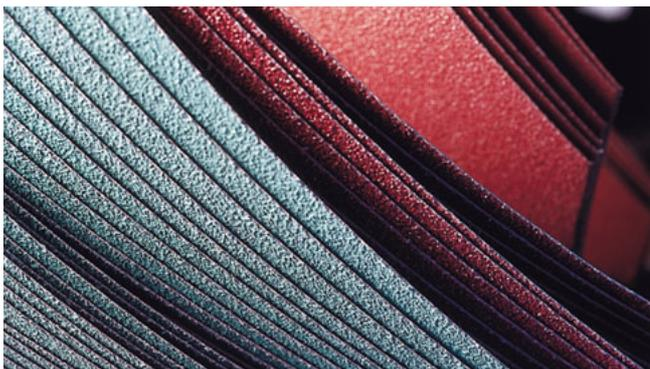
Coated abrasives are made by bonding natural or synthetic abrasive particles onto a flexible backing, which can be cut into different shapes (belts, discs, sheets) for use in a wide range of surface treatment and polishing applications, on markets ranging from home renovation to the metal working industry.
