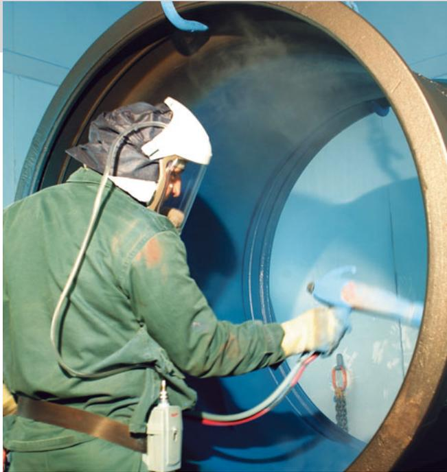
Epoxy paint coating for wide-diameter pipe in ductile cast iron.
